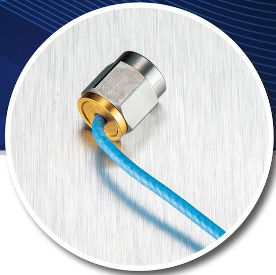
InstaBend® 047 are flexible coaxial microwave assemblies designed for interconnects between RF circuit cards, medical equipment, and enclosure panels. This cable's low profile and flexure allows for bending close behind the connector which simplifies cable routing. IB-047 assemblies are available in a variety of lengths and connector types, making them a versatile solution for a wide range of applications.
