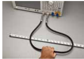
Cable is pulled off center 10" in both directions
