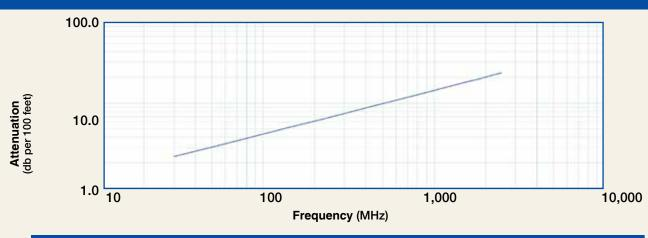
Calculate Attenuation = (0.424232) • FMHz + (0.000563) • FMHz (interactive calculator available at http://www.timesmicrowave.com/cable\_calculators)
