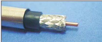
5. Place the connector onto the cable. Twist the connector back and forth as it is pushed onto the cable. Push the connector until it comes to a hard stop. Slide the ferrule up and make an impression in the excess braid as a mark for trimming.
