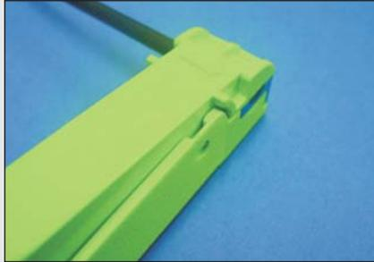
3. Debur the center conductor using the debur tool. A half dozen back and forth motions by hand or 3 seconds of clockwise motion in a low speed drill will be sufficient.
