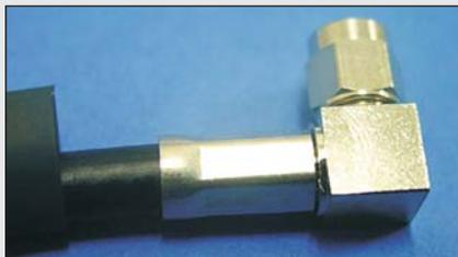
7. Slide the shrink boot towards the connector as far as it will go, and shrink it down using a heat gun until a lip of adhesive is visible at each end of the boot.
