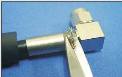
6. Using a 0.255 inch hex crimp die, crimp the ferrule as close to the connector body as possible. Do not double crimp.
