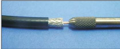
4. Place the shrink boot and ferrule over the end of the cable and fold the round wire braid away from the outer conductor.
