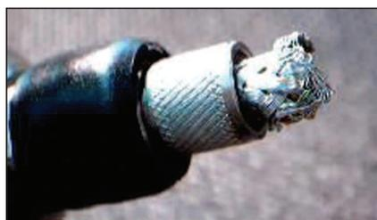
▲ Fig. 4 Failed cable attachment.
