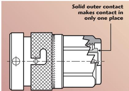
▲ Fig. 2 Connector with solid outer conductor contact.
