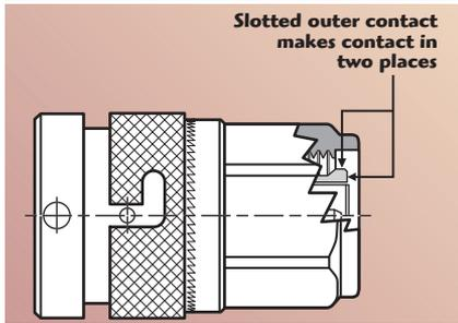
▲ Fig. 1 Connector with slotted outer conductor contact.
