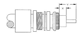
STEP 8. Install Body & Strain relief boot.
