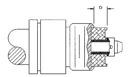
STEP 2. Expose conductor. A = 0.250"
