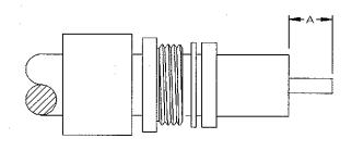
STEP 5. Flare out braids but do not comb them out. Trim braids to shoulder of ferrule. Trim core back to this dimension:  $X = 0.115^{\circ}$  Trim conductor back to this dimension:  $Y = 0.350^{\circ}$
