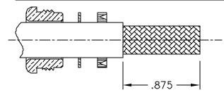
Trim cable jacket to dimension shown. Slide clamp nut, washer, gasket and clamp onto cable as shown. Cable jacket should bottom on step in braid clamp.
