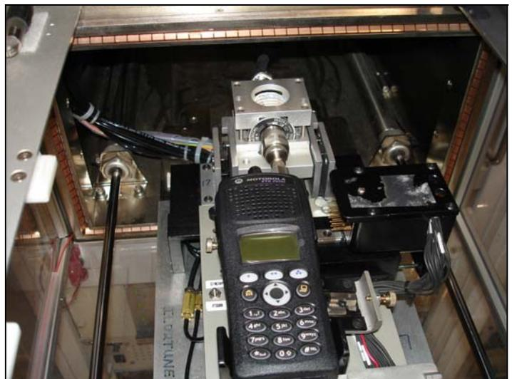
(Radio during test. Semi-automatic test station)
