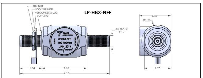
All LP-HBX-N Series connectors are labeled "Surge" and "Protected". The "Surge" side must be connected to the expected surge source (e.g. antenna). The "Protected" side must be connected to the equipment. *Protector and equipment damage can occur if the protector is installed backwards.*
