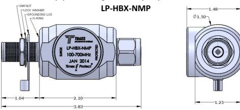
The NMP version has an **N** connector, **M**ale gender, on the **P**rotected side
