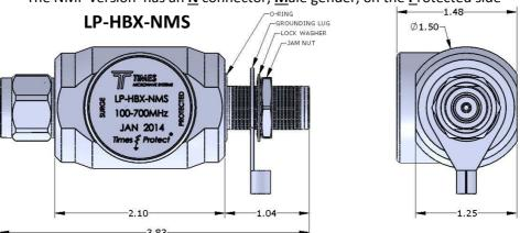
The NMS version has an  $\underline{\mathbf{N}}$  connector,  $\underline{\mathbf{M}}$  ale gender, on the  $\underline{\mathbf{S}}$  urge side. Except for connector gender, all HBX protectors have the same mechanical and electrical specifications. All protectors are weatherized and sealed to IP65 allowing for outdoor as well as indoor installation.
